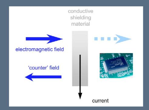
Electrical conductivity is a prerequisite for an EMI shielding material. This is due to the physical phenomenon that electric fields and varying magnetic fields induce currents in the electrically conducting shielding material. In turn, these currents generate counteracting fields which weaken - or in the ideal case cancel - the originally applied fields. Ideally, external fields stay outside the shielding material, and internal fields stay inside.
