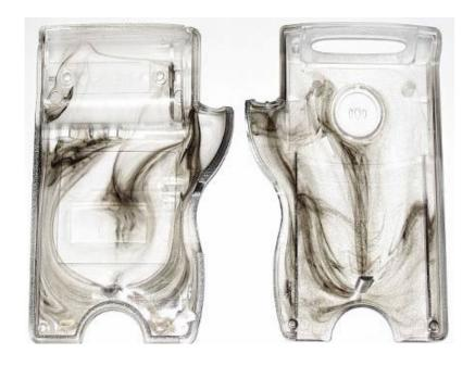
To **minimise shear** during filling of the part mould, it is advisable to avoid sharp corners in plastics parts, and to try to ease the flow by replacing the sharp corners by rounded ones. As part of the effect of shear stress in the part, on the design stage we have to minimise the sharp corners, giving them generous radii to expedite flow of the conductive melt.
